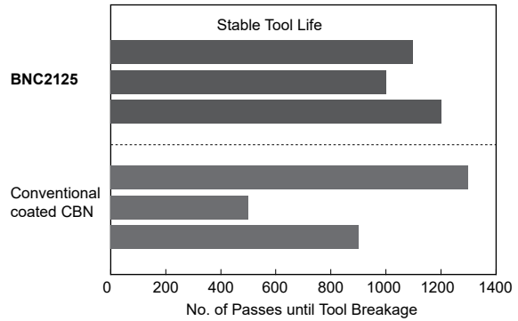
Interrupted Cutting of Hardened Steel
