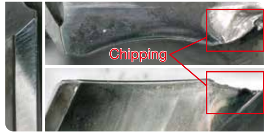
After drilling 1,000 workpieces (5 holes per workpiece)
