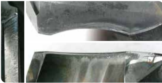
After drilling 2,500 workpieces (5 holes per workpiece)
