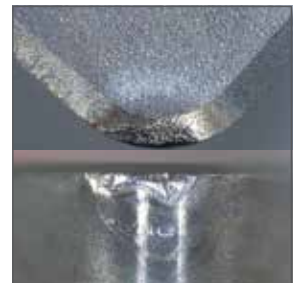
Competitor (uncoated) (After cutting 45 km)
