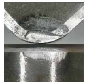
Conventional Tool (uncoated) (After cutting 0,5 km)
